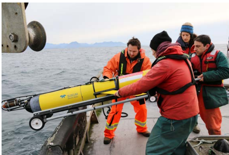
A glider equipped with a hydrophone is deployed to listen for and identify whale songs.
